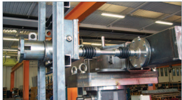
Stainless steel drive extensions for remote location of ISO 13628-8 rotary torque tool receptacle.
