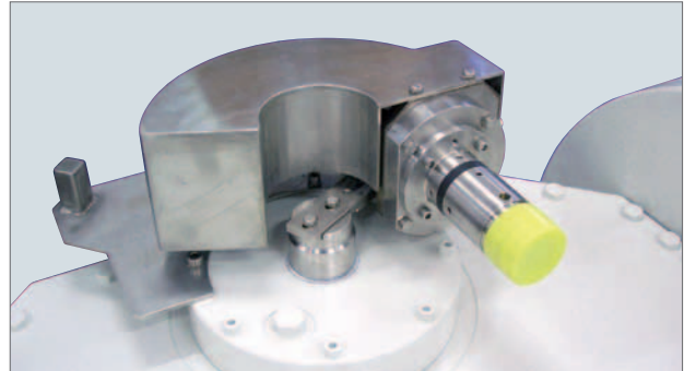
Position transducer assembly with electrical instrumentation connector.
